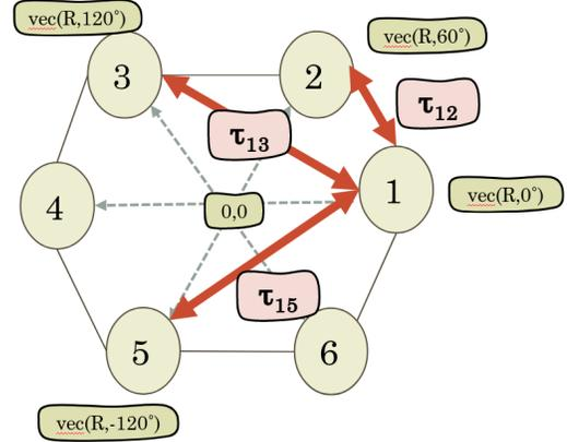
Fig. 1: In this example the center of formation is  $(0,0)$ . Relative to the centre,  $\tau_1$  for agent 1 can be represented in polar coordinates as a vector with magnitude  $R$  and direction  $0^\circ$ . Similarly,  $\tau$  direction for agents 2, 3 & 5 can be encoded with  $60^\circ$ ,  $120^\circ$  &  $-120^\circ$ .  $\tau_{rel}$  for each agent can be seen for  $\tau_{12}, \tau_{13}, \tau_{15}$
