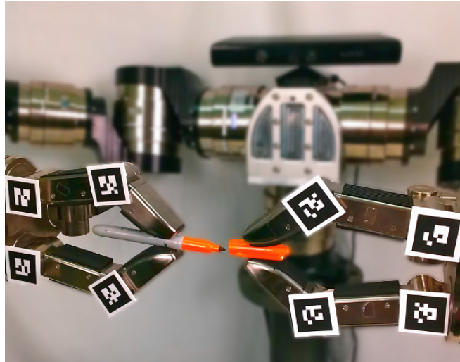
Fig. 1. Bimanual Schunk LWA4/SDH capping a pen using visual feedback from online camera registration and end-effector tracking.
