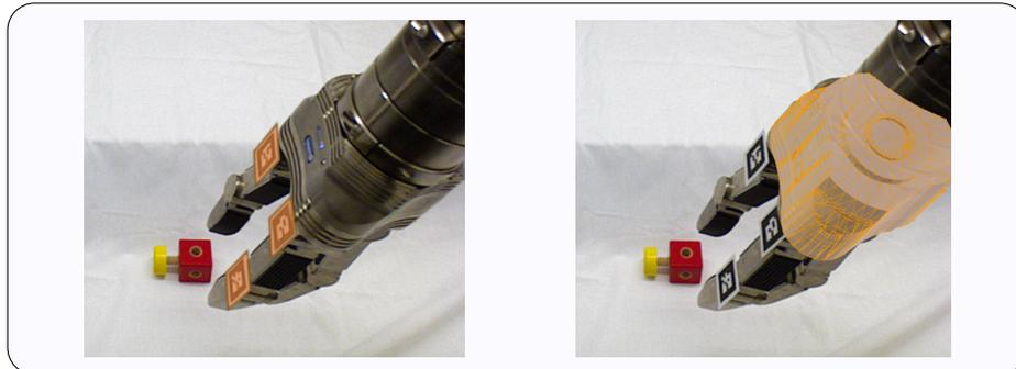
**Fig. 3.** Marker-based tracking (left) and model-based tracking (right).
