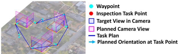
Fig. 1. Given the inspection tasks, a high-level task plan is derived by solving an energy-efficient TSP problem.
