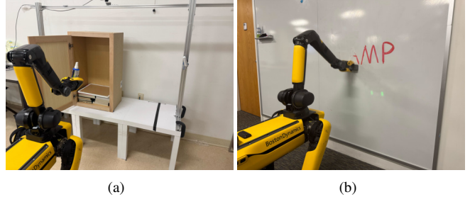
Fig. 1. A Boston Dynamics Spot ® robot demonstrating skills that must be composed to solve long-horizon hybrid robot planning problems. Fig. 1(a) shows the robot in the process of executing a kinematic skill (Pick) to pick up a spray bottle. In Fig. 1(b), the robot uses a non-kinematic skill (Erase) to maintain force-controlled contact while erasing a whiteboard.
